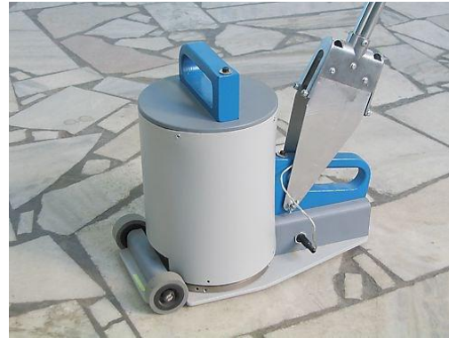
Holographic subsurface radar RASCAN-4/2000in work.
