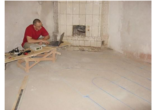
Holographic subsurface radar RASCAN-4/2000in work.
